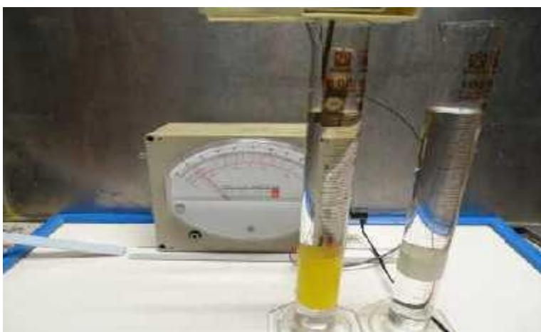
FIG. 2. This is a simple but high input resistance analogue conductance meter that actually measures current in micro ampere/h and seen measuring the conductance of nano metre silver in water in a 100 ml flask. The actual measurement reads about 12 micro ampere/h for the sample of colloidal silver. The input resistance is 10, 000 million Ohm and operates at a potential of just 1 volt direct current, to ensure it will remain well under the equilibrium voltage of water at 1.23 volt DC. The other 100 ml flask is filled with pure water and reading just 2 micro ampere.
