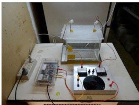
*Figure 1: This show the entire set-up, i.e. The 300 Volts DC @ 50 micro ampere (limited) power supply unit to the left, the actual measuring instrument at the bottom right and a 10 litre tank filled with 9 litres of deionised water and containing two pure silver electrodes at the rear.*
