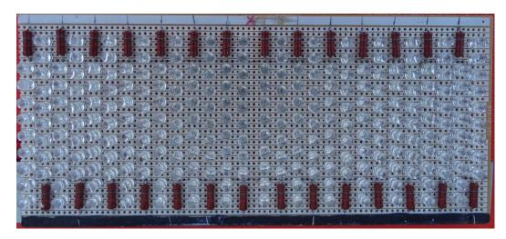
Matrix of 28 parallel rows of 9 violet LEDs wired in series making for 252 LEDs on an area of 250x100mm OCB. Instead of having rows of 10 at 3.5 volt =35 volt, columns of 9 allow for 4 volt per LED = 36 volts in total and within the limit set by the LM317T voltage regulator.
