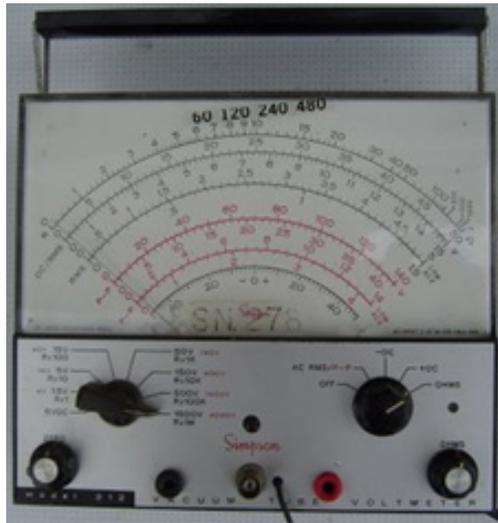
Illustration of a typical vacuum tube voltmeter. Please note that the values increase to the right and diminish toward the left in an opposite way to conventional analogue multimeters. To the far right is the maximum value of 1,000 million Ohm shown.
